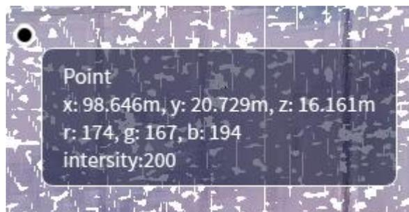
Click "**Distance Measure**", left-click on two points in the point cloud, and the distance between the selected points will be displayed for measurement. If multiple points are clicked continuously, the distance of continuous line segments between multiple points will be measured. To undo a selection, right-clicking the mouse will undo the previous selection.
