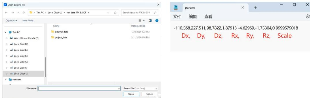
If you do not have the seven parameters, you can calculate them based on the existing control points. Click "Calculate" to open the seven-parameter calculation interface.
