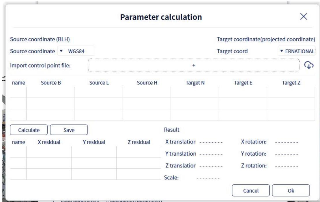
Click the "Import File" button to import the control point file needed for calculating the seven parameters. The file format supports ".csv" or ".txt" formats. The specific data includes: Point Name, Latitude (degrees:minutes:seconds) [e.g., 121:32:11.235], Longitude (degrees:minutes:seconds), Elevation, Projected Plane Coordinate X, Projected Plane Coordinate Y, and Elevation.
