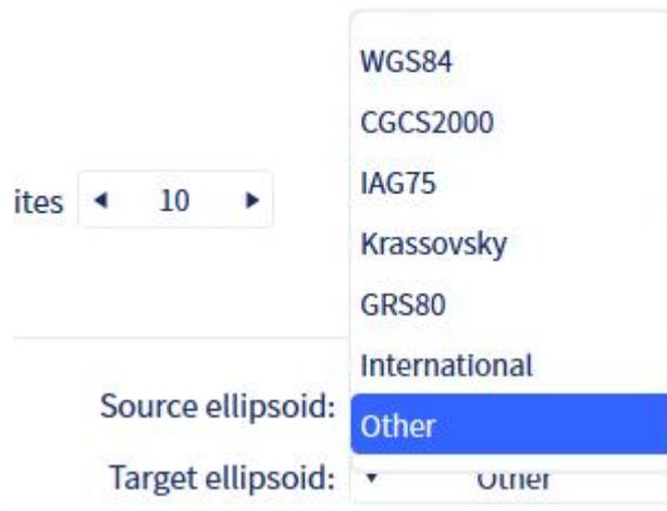
When users select a custom ellipsoid, they need to input the ellipsoid's semi-major axis (a) and 1/f (where f is the ellipsoid flattening).
