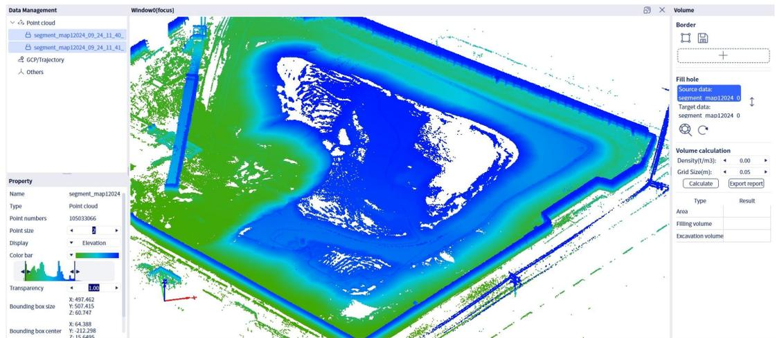
After importing the data, the interface on the left will display the pile calculation window. Similar to the pile calculation function, the pile comparison requires users to perform boundary selection, reference surface setting, meshing, hole filling, and other operations separately for the two sets of point cloud data.
