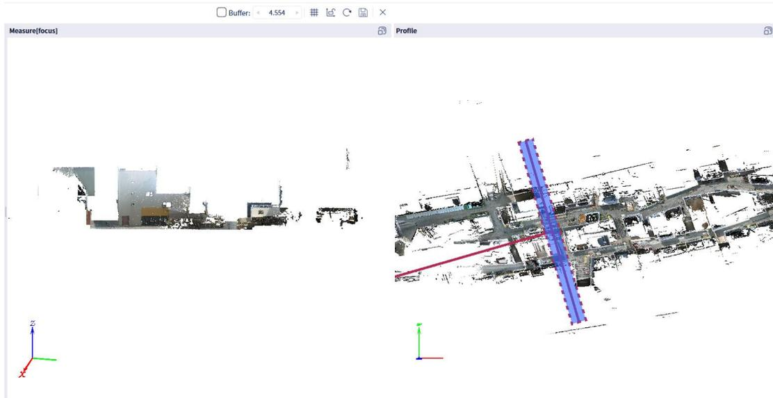
In the main point cloud display window on the right, click and move the mouse to select the point cloud data you want to view in cross-section. Once you have made your selection, double-click to display the selected point cloud data in the cross-section window on the left. While moving the mouse to select points, users can also set a fixed width in the buffer area to select the point cloud data they need to view.
