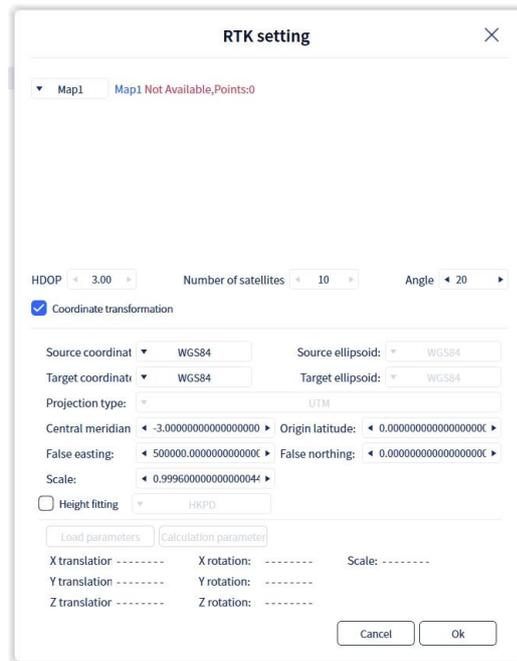
If you need to perform coordinate transformation on the acquired data, make sure to check the coordinate transformation box. Be sure to select the **source coordinate system**, **source ellipsoid**, **target coordinate system**, **target ellipsoid**, central meridian (degrees), east offset, and latitude origin (degrees) according to the actual situation.
