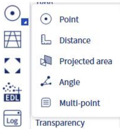
Click "**Point Measure**", left-click on a point in the point cloud, and the information of the selected point will be displayed, including point coordinates, point cloud color RGB information, intensity signal, etc. Note: Only when the point cloud has the above information during scanning can it be displayed.
