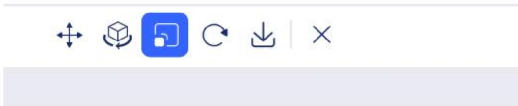
Click the tool and the software will display a bounding box around the current point cloud data, with the scaling arrows for six directions enabled. You can perform clipping option for a single point cloud layer or multiple layers at once.
