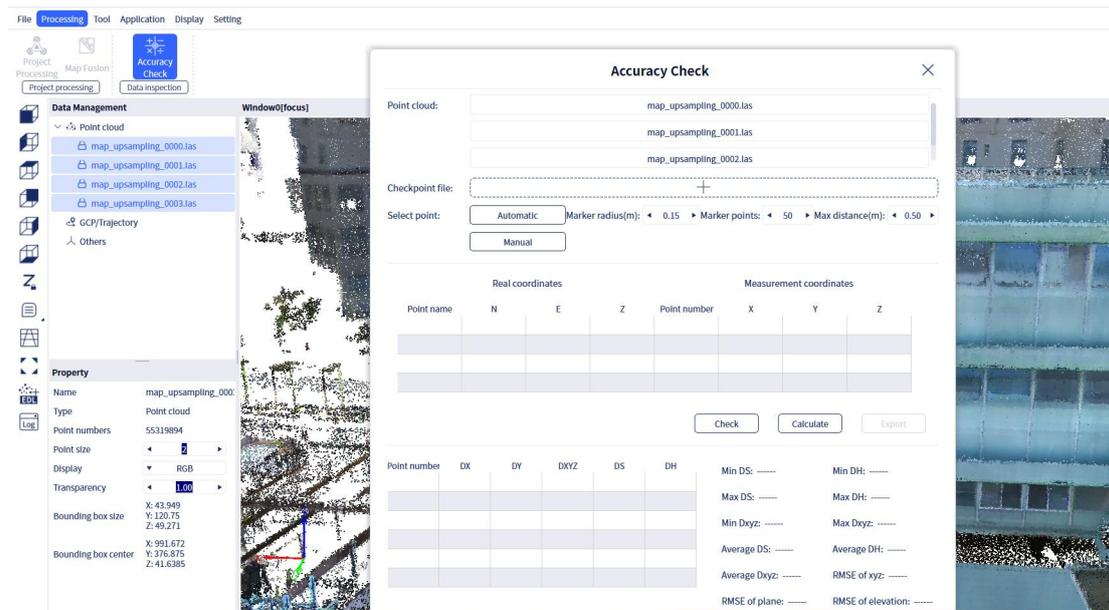
If you have scanned reflective targets (at the checkpoints) during data collection, you can click the auto-selection function, and the software will automatically extract the coordinates of the target center points. The auto-selection function provides three parameters:
