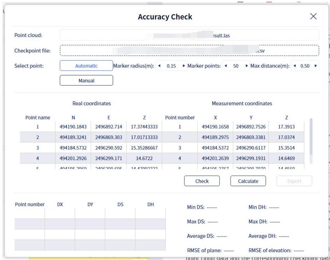
The software supports Accuracy Check for individual point clouds as well as for multiple data sets enhanced by L2 Pro. In the left data panel, select the multiple data sets that need accuracy verification simultaneously, and click "Accuracy Check" in the toolbar to perform verification on multiple data sets.
