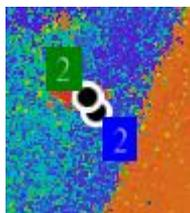
Left-click in the point cloud to select the checkpoint location, and the selected point will be labeled with a green tag by default. [Note: The software will automatically search for the true value points near the selected point and automatically display the tag for that point.]
