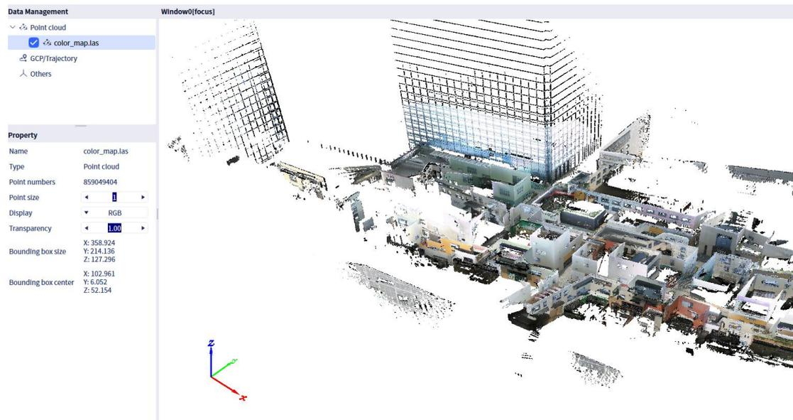
Selecting "Intensity," "Elevation," or "GPS Time" will display the point cloud using different color bands. The software provides various color bands for these display modes, and users can choose the color band according to their needs.
