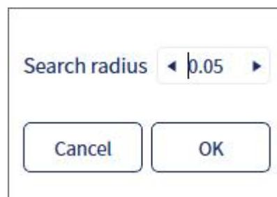
Theoretically, the larger the search radius, the smoother the resulting point cloud will be. However, for structured point cloud data, it is recommended to perform smoothing with the default parameters.
